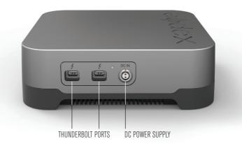
Connect the included DC power supply to the DC IN connector of the Capture Drive 2.0 Dock. There are two Thunderbolt Ports available - connect the port on the right side to a Mac computer that has the required Codex software installed.
