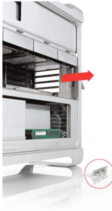
Remove the PCI blanking plate for the slot you intend to use for the ATTO SAS card. Do not move the system graphics card that is already installed.
