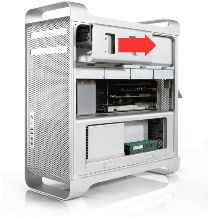
Disconnect the power and ribbon cables from the optical drive and remove the carrier fully.
