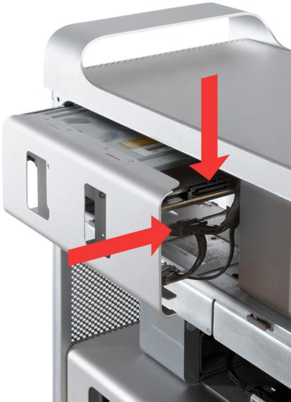
Fit the System Drive into the spare slot of the Optical Drive Carrier using the instructions that came with the specific Optical Bay HDD Mount Kit being used. This will normally require use of the side mount holes:
