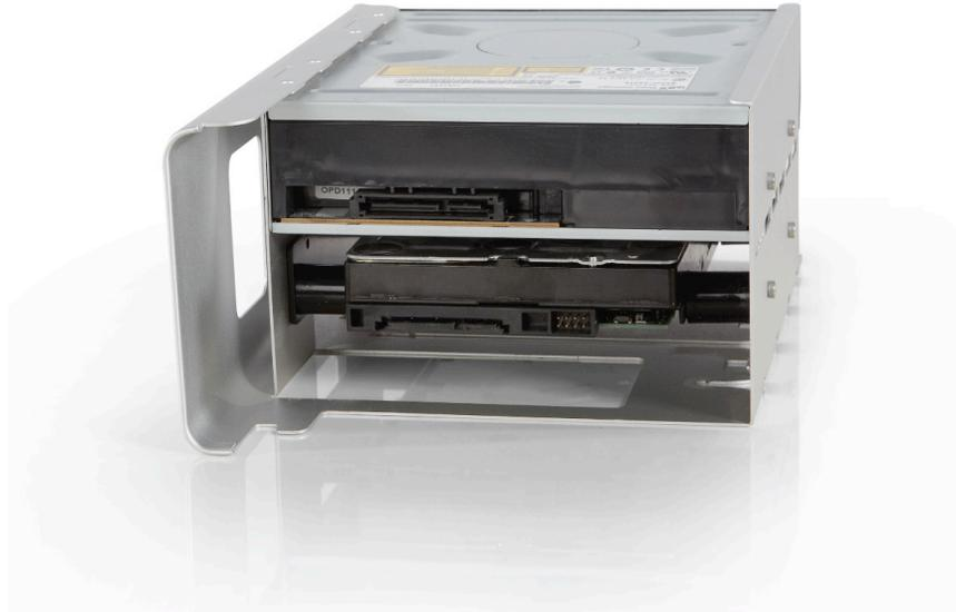
Then slide the optical drive carrier halfway back into the drive bay and reconnect the power and ribbon cables.
