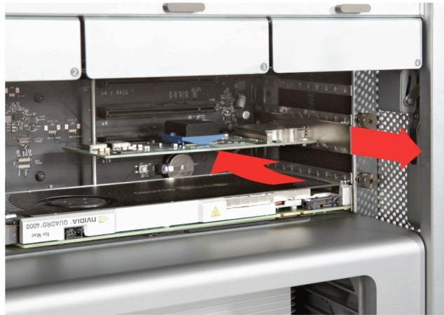
First remove the PCI blanking plate
